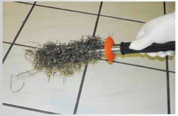
Move a magnet inside a stainless round bar up and down and the highly adhesive magnet attracts metal swarf. Then pull the button-swarf fall down
